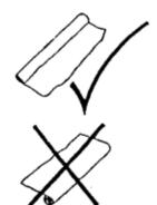
The rolled liner bags must be placed so that they roll from underneath.
